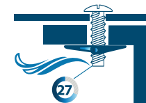
Thick flange predrilled, inwards
