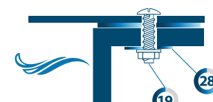
Thick flange predrilled, out
